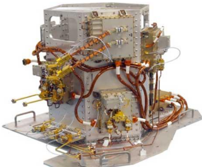
Above: The Global Microwave Subsystem imager receiver, with the channels completed. This equipment will receive the microwave signals after they bounce off clouds and the surface. Image courtesy of NASA.
